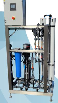
range. Only one HP pump is necessary to ensure pressure sufficient for the proper operation in series of the 2 stages. Combining simplicity and compactness, the **Bi-Osmeo Eco**
